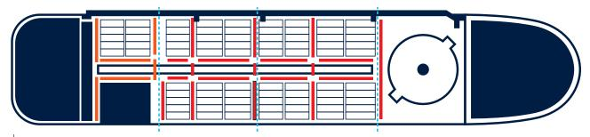
Example of an FPSO seen from top showing typical locations for fire- and explosionsafe drain gullies (red/orange lines) and flexible fire walls (blue dots).
